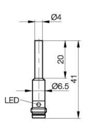
Inductive Sensors BES 516-3017-E5-C-S49 D4 x 41 normally-closed Sn=0,8mm shielded
